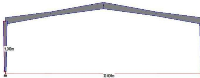
Fig -3.1: Elevation PEB frame
