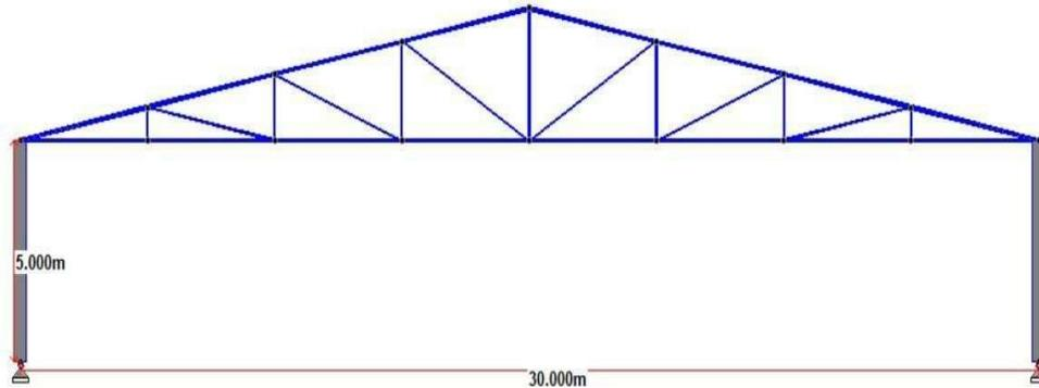
Fig-3.3: Elevation of conventional steel frame
