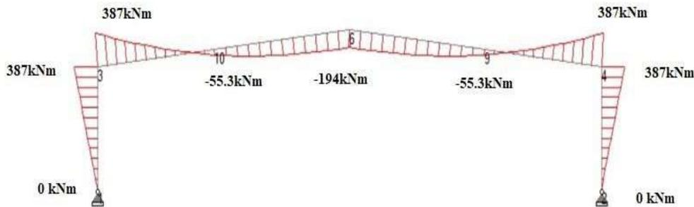
**Fig 3.2: Bending moment diagram**
