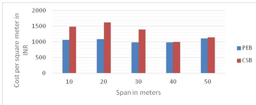
**Fig -4.3: Cost of structure per square meter**
